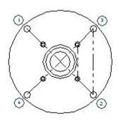
NOTE: WHEN ATTACHING THE GRINDER TO THE ADAPTER PLATE AND THE ADAPTER PLATE AND CHASSIS TO THE HOUSING, USE A CROSSING PATTERN WHEN TIGHTENING CAP SCREWS AND NUTS. SEE FIGURE AT LEFT
