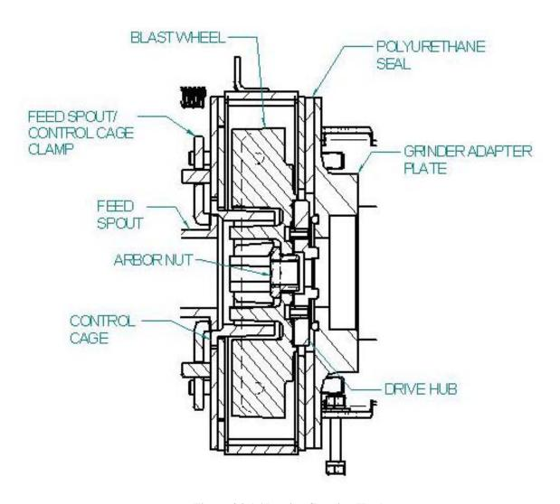
Figure 4.2.1 Abrasive Cleaning Head
