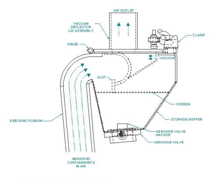
Figure 4.5.1 Rebound Chamber - Deflector Plate - Hopper
