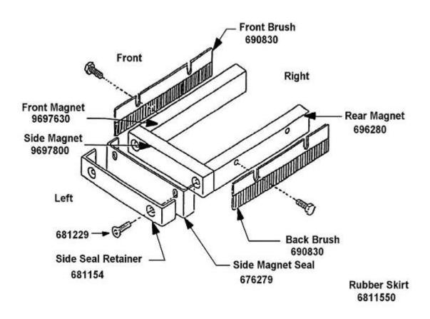
This magnet and seal illustration shows how the machine is set during the right side edging mode. This is achieved by simply removing the right side retainer, right side magnet seal and the right side magnet. For normal (non-edging) operation, the right and left side arrangements are identical. For left hand edging, reverse the above arrangement from right to left.
